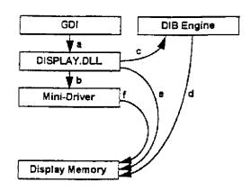
a) GDI loads DISPLAY.DLL as the primary display driver. If no mini-driver is installed, the display is run as EGA or VGA.
